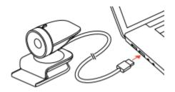
$\ensuremath{\text{1:}}$  Connect the USB cable from the P5 USB to the USB A port on your computer.
